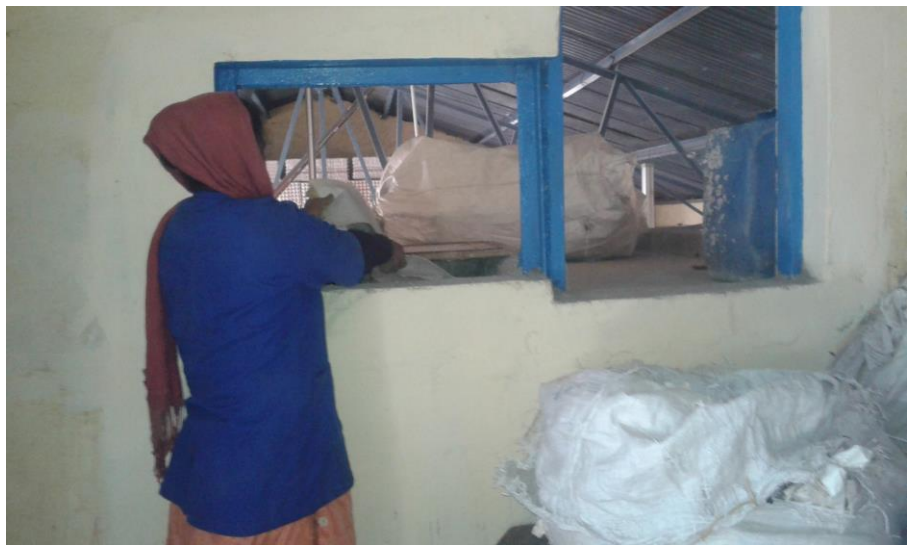
Putting waste paper in the Hydra-pulper machine →
